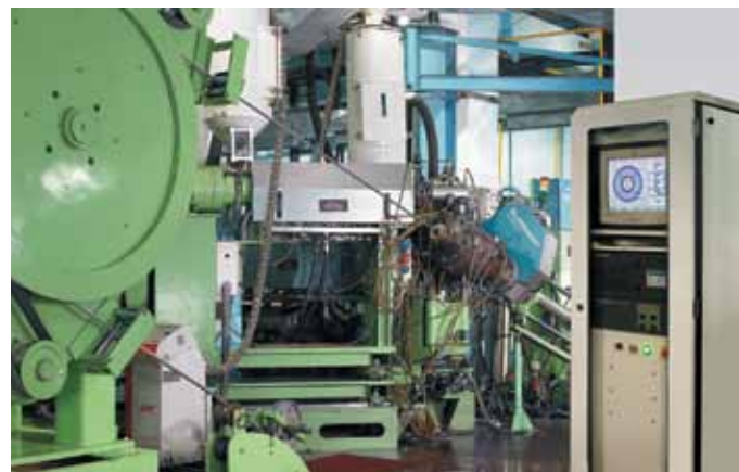
Figure 2 : THREE LAYER COMON TRIPLE EXTRUSION METHOD
